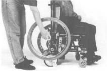
Put the wheelchair plus scalamobil in a parallel position; tilt the entire mechanism slightly backwards and balance it out. You have reached a balanced position when you feel no pressure at the handles, neither forward nor downward. Then advance the scalamobil to the edge of the stairs until
