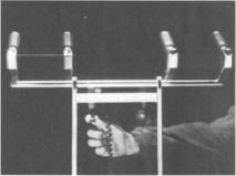
In such case pull out the indexing bolt somewhat to move the handle to the right or left until the bolt catches.
