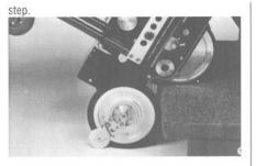
Then the outer wheels follow and the second part is accomplished when both pairs of wheels are securely on the next step in a parallel position.
