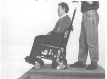
To remount the wheelchair's wheels, lift the chair with the scalamobil's outer pair of wheels and put the chair's wheels back into its fixtures. Always make sure that the full floating axle system locks securely.
