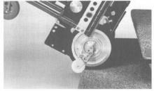
If the steps have a high depth, the climbing process may have to be interrupted. Release the rocker switch and advance the scalamobil- wheels in parallel position - forward to the edge of the next step.
