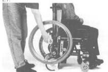
Put the wheelchair plus scalamobil in a parallel position; tilt the entire mechanism backwards and balance it out. You have reached a balanced position when you feel neither pressure downward nor for-
