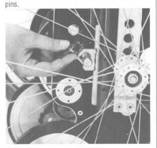
Attention! Never replace the locking pins with nails, screws or the like. Only use the original Alber locking pins.
