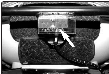
Fig. 7. Disconnecting the cables
