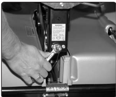
Fig. 52. Turn counterclockwise to raise the seat lift.
