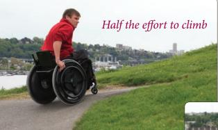
Similar to bicycle technology, low gear gives added capability to ascend inclines, negotiate uneven terrain and go places that were previously challenging.
