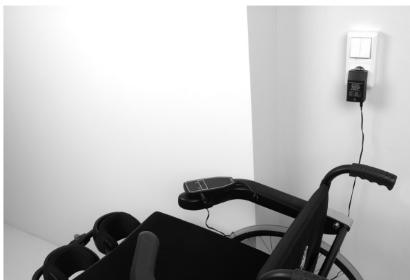
The charger cable is connected to the control panel.
