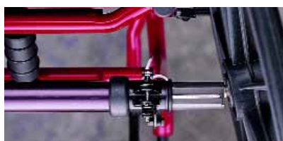
Camber-bar technology provides quick and easy camber changes; each insert provides two camber choices.
