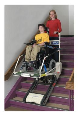
Super-Trac is simple to use. As shown in this sequence, a small operator can easily transport a passenger in a heavy power wheelchair up and down stairs. Above, the passenger has boarded the platform using the integrated ramp. The wheelchair is being secured using four adjustable tie-down straps. An electrically interlocked seat belt provides additional passenger security.
