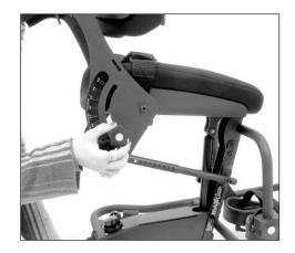
To adjust the seat, depress the spring button on the adjustment tube and move (up to three increments) in the intended direction.
