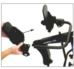
**3** Place seat assembly onto base. As shown. Tip the seat assembly forward and insert seating system tab into slot.
