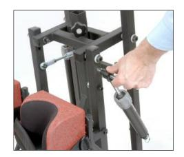
**14** If you ordered the table option, remove the grab bar/front pad bracket and insert the table sleeve. Replace the standard knob with the longer studded knob, be sure the slot lines up with the tightening knob.
