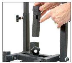
**15** Remove the glide handles and insert the table with frontpad into the bracket. If desired, re-insert glide handles.
