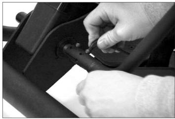
**#18** If you ordered the removable actuator handle it can be removed by loosening the knob as shown.
