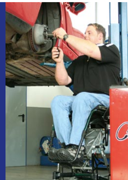
Flexible and quick seat height adjustment – supported by gas springs
