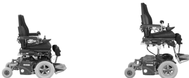
Fig. 67. Moving the seat by adjusting the height of the seat.
