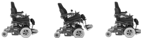
Fig. 43. Movement of the seat when adjusting the angle of the seat.
