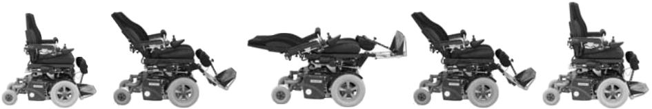
Fig. 69. Movement of the seat when adjusting the leg rest/back rest.
