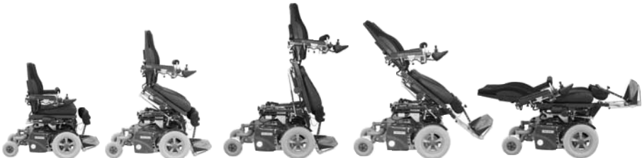
Fig. 71. Movement of the seat during vertical/horizontal adjustment.
