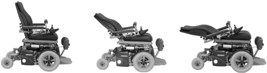
Fig 53. Back rest slope.
