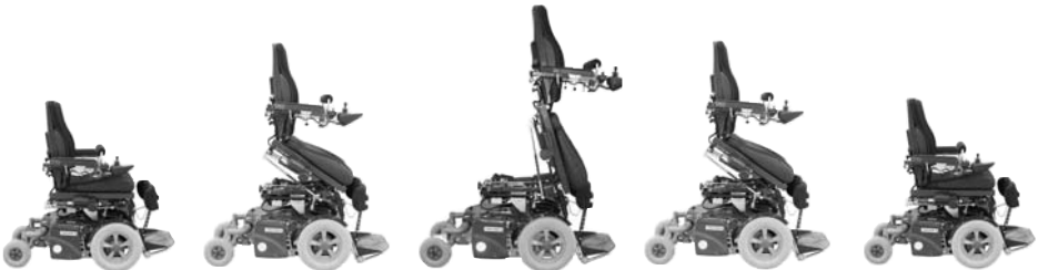
Fig. 73. Movement of the seat during standing
