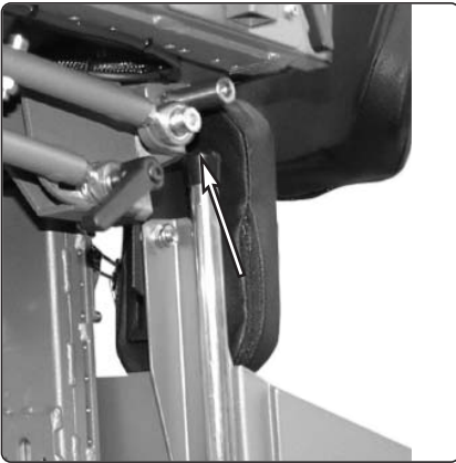
Fig. 1. Swivel rod head, viewed from under the seat, right side.
