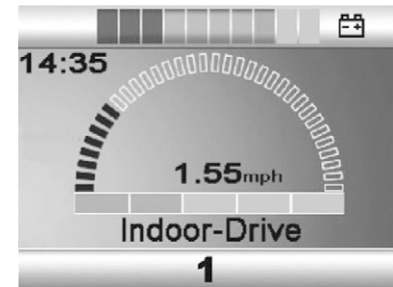
Figure 65. Standard display image with speed indicator.
