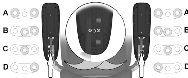
Figure 27. The endpoints are set by moving one or two screws between three different positions underneath the arm rest.
