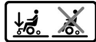
Figure 130. The support wheels must always be fitted when you drive.
