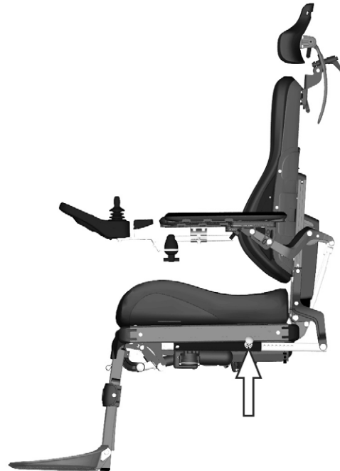
Figure 17. Manual clamp Tube for the Backrest Recline
