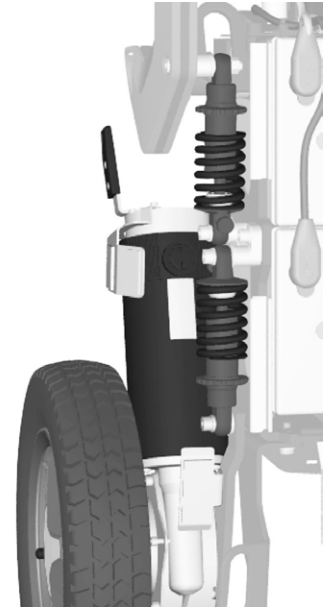
Figure 2. Drive package and shock absorbers.
