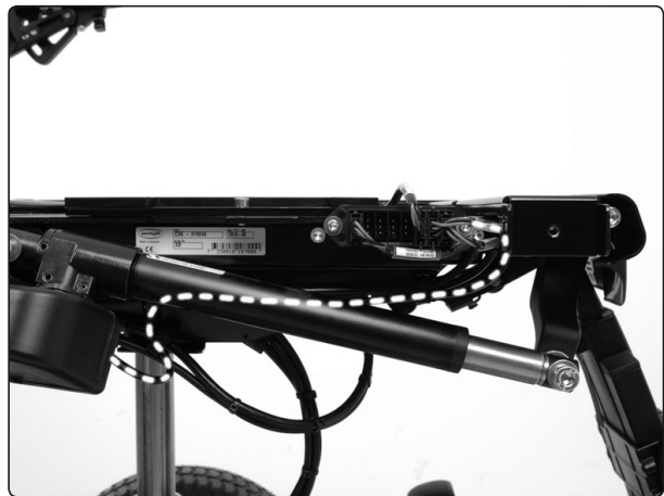
The actuator cabling is connected to the contact block on the right side of the seat
