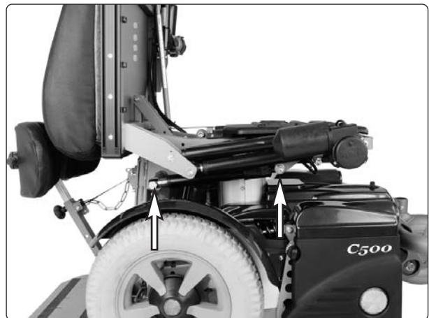
The back rest angle actuator is mounted with two screws.
