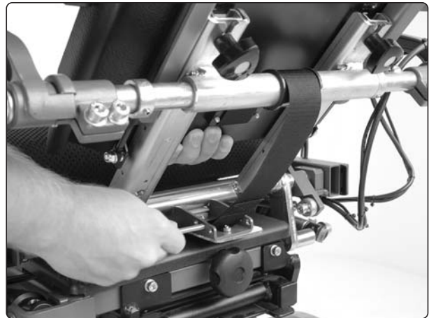
Carefully lift the back rest up until the strap slackens, and pull out the cotter.
