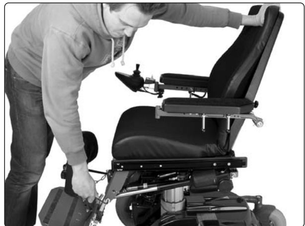
Push the back rest backwards as the actuator is removed
