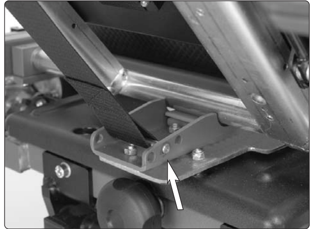
Circlip on the right side of the lower strap bracket.
