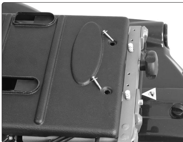
Mounting of crush protection cover
