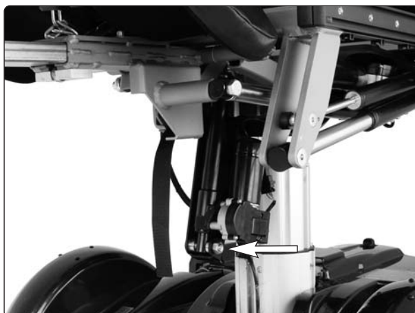
Lower fixing for seat angle actuator.
