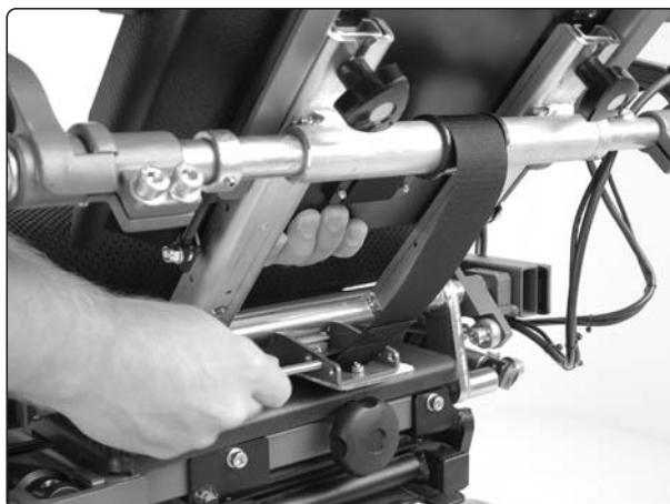
Carefully lift the back rest up until the strap reaches the lower bracket and fit the cotter.
