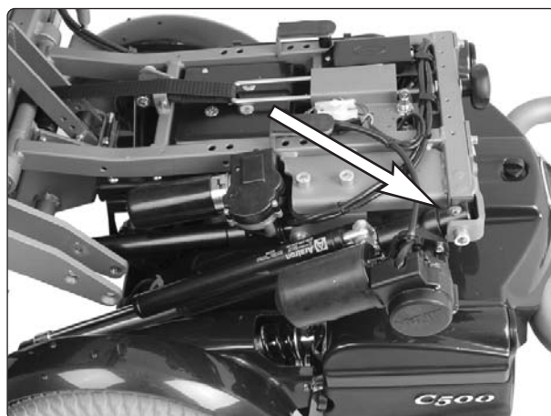
Rear fixing screw of the actuator.
