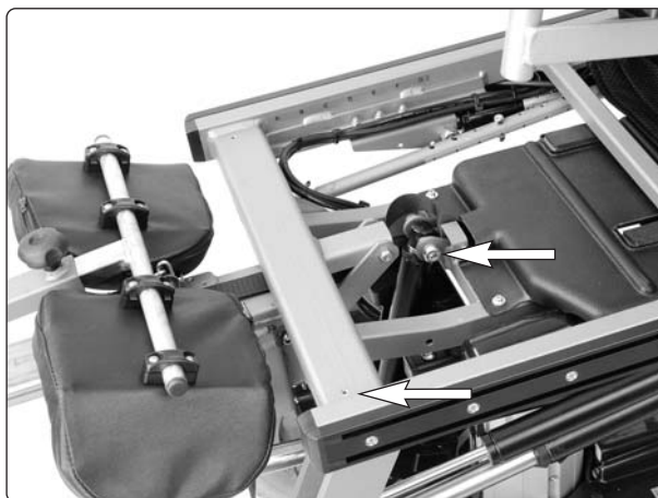
Upper fixing for seat angle actuator.
