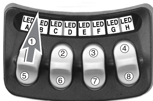
Stand the seat to its upper position, move and hold the toggle switch towards position 1 until the Stand Actuator movement stops.
