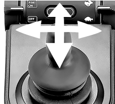
Figure 60. With the use of Bluetooth® the joystick can take control of the mouse functions.
