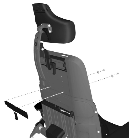
Figure 482. The locking mechanism is held in place by two screws.
