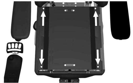
Figure 476. The seat plates are held in place by two screws at the back edge and two quick-mount clamps at the front.
