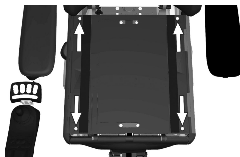
Figure 10. The seat plates are held in place by four screws.
