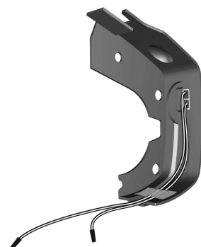
Figure 434. The front turn signal is assembled on the drive package cover.
