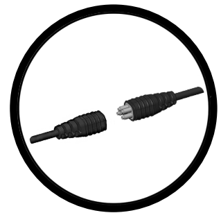
Figure 120. The control panel's cable connection is in most cases located under the armrest.
