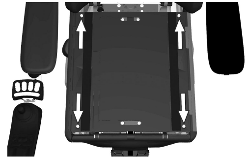
Figure 193. The seat plates are held in place by four screws.
