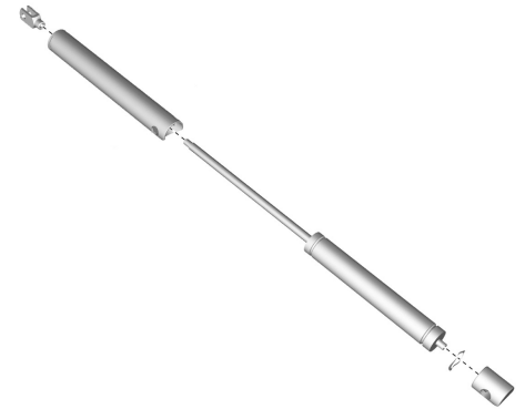
Figure 324. The rear and front bracket is screwed on to the gas spring.
