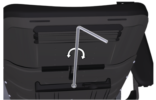
Figure 486. Use the supplied adjustment crank.
