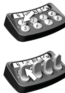
Figure 282. The ICS switchbox has two versions, one with buttons and one with paddle switches.
