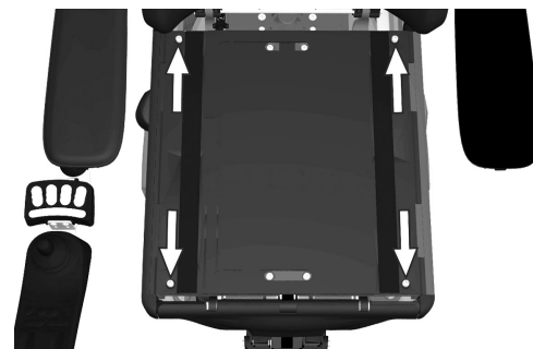
Figure 27. The seat plates are held in place by four screws.
