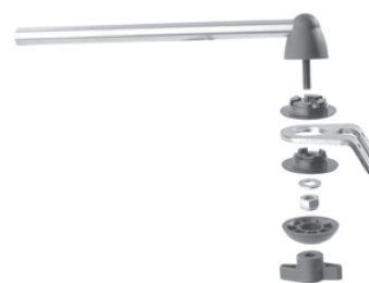
Figure 503. Exploded view of the panel holder's joint.
