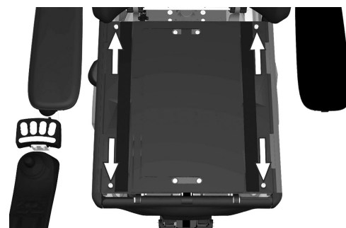
Figure 480. The seat plates are held in place by two screws at the back edge and two quick-mount clamps at the front.
