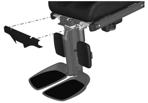
Figure 195. Remove the leg rest's top cover by carefully pulling it straight out.
