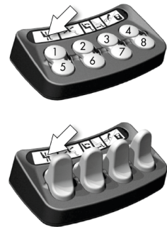
Figure 287. The ICS switchbox has two versions, one with buttons and one with paddle switches.
