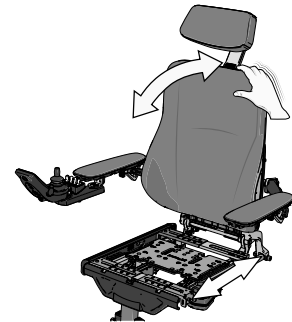
Figure 75. Push the backrest forward and then pull it backwards.
