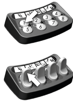
Figure 286. The ICS switchbox has two versions, one with buttons and one with paddle switches.
