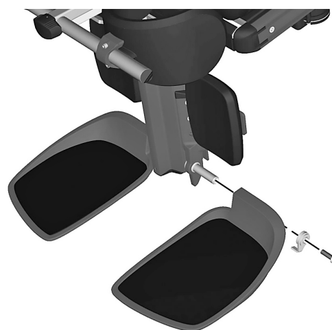
Figure 161. The footplate and its friction brake.
