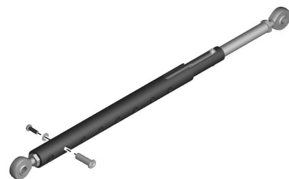
Figure 494. Remove the screw fixating the length setting of the parallel armrest rod.
