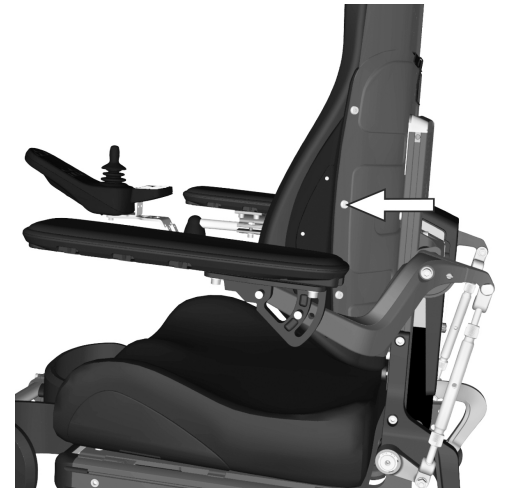
Figure 524. The trunk support height is fixed using one screw.
