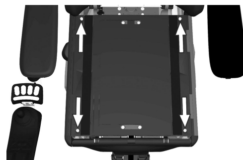
Figure 500. The seat plates are held in place by two screws at the back edge and two quick-assemble clamps at the front.
