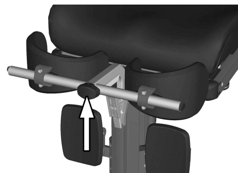
Figure 549. Adjusting the knee support depth.
