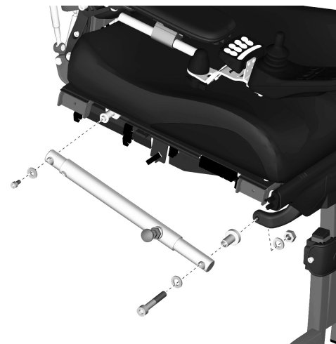
Figure 151. The manual leg rest adjustment unit is held in place by two screws.
