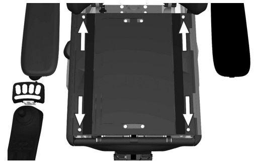
Figure 210. The seat plates are held in place by four screws.
