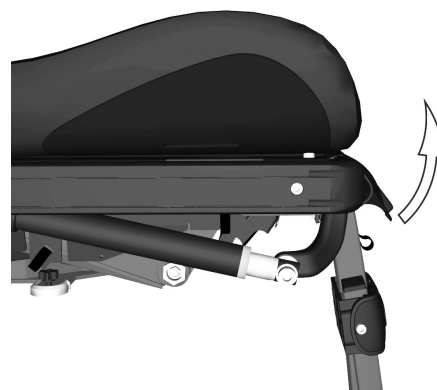
Figure 136. Lift up the leg rest's top cover.
