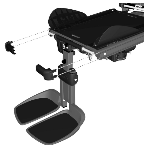
Figure 127. Reassemble the front ends of the UniTrack rails.
