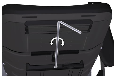
Figure 513. Use the supplied adjustment crank.
