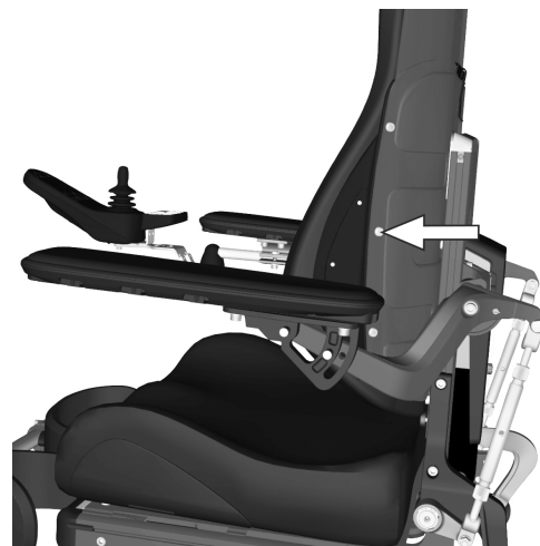
Figure 547. The trunk support height is fixed using one screw.
