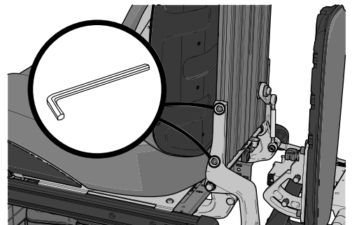
Figure 94. The backrest profile is secured by two screws on the left and right.
