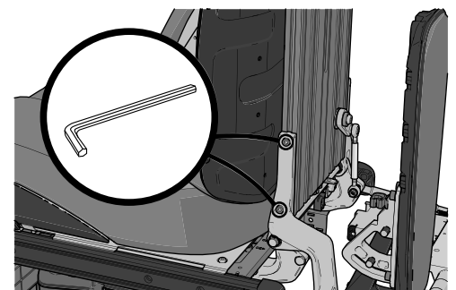
Figure 101. The backrest profile is secured by two screws on the left and right.
