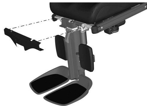
Figure 148. Mount the leg rest's top cover by carefully pressing its bracket into place on the leg rest's fixing screws/spacers.
