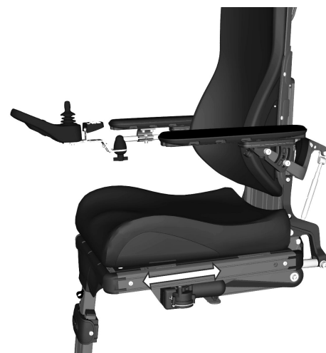
Figure 548. The position of the thigh support can be adjusted.
