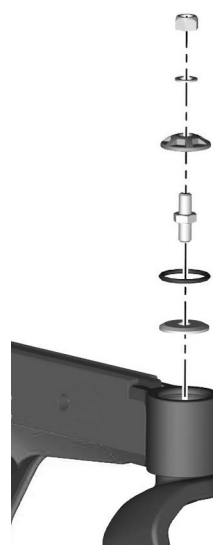
Figure 439. An early revision of the friction brake.
