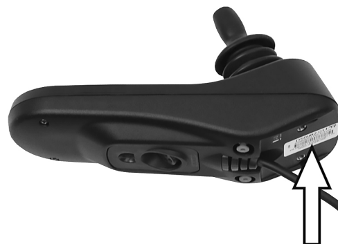
Figure 8. Control panel ID number.
