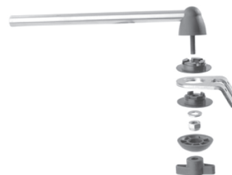
Figure 528. Exploded view of the panel holder's joint.
