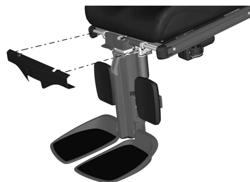
Figure 143. Remove the leg rest's top cover by carefully pulling it straight out.
