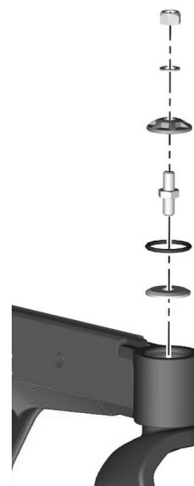
Figure 422. An early revision of the friction brake.
