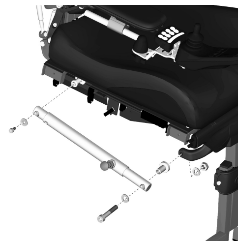
Figure 150. The manual leg rest adjustment unit is held in place by two screws.
