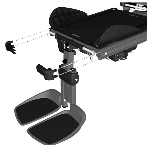
Figure 124. Remove the front ends of the UniTrack rails.
