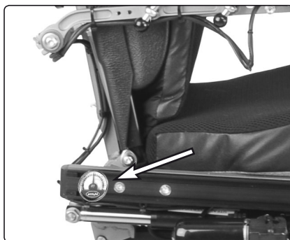
Mounting the angle gauge.
