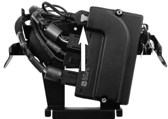
The control panel cabling is connected to the Power Module.
