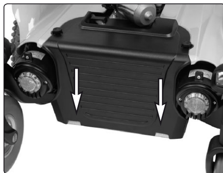
The front cover is fitted on the front edge of the chassis.
