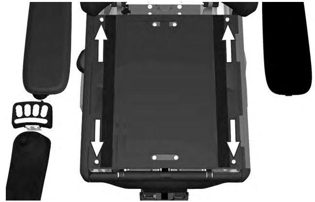
Figure 248. The seat plates are held in place by two screws at the back edge and two quick-assemble clamps at the front.
