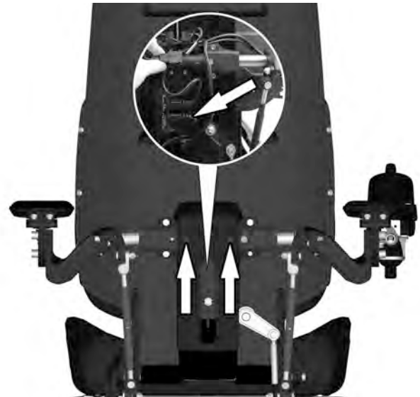
Figure 182. Reconnect the Rnet cable from the contact block at back of the back rest.
