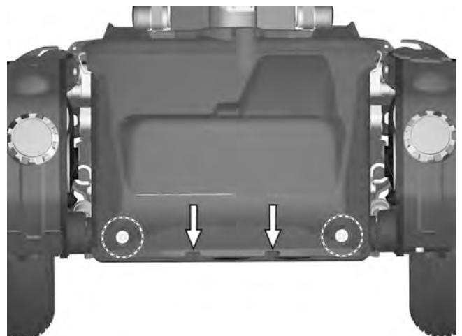
Figure 10. The chassis front cover is assembled partially inside the chassis at the lower edge.
