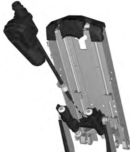
Figure 125. Assemble the actuator to the sleigh by unscrewing its nut.
