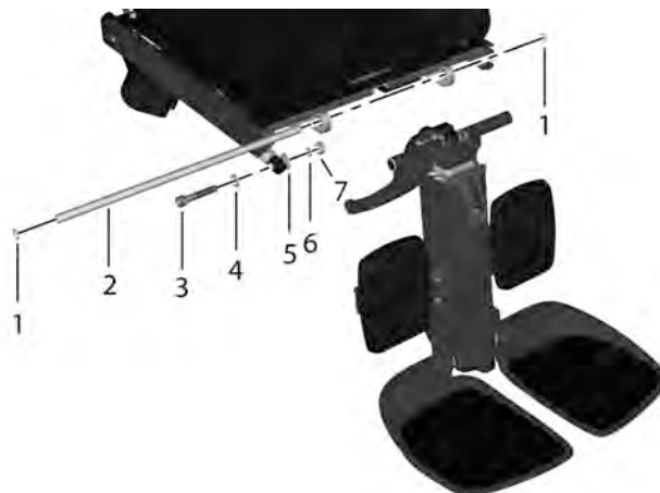
Figure 232. The legrest is held in place by an axle (2) with a circlip (1) on the left and right hand side of the legrest.. The front bracket of the actuator is held in place by a screw (3), washer (4) and shim washer (5) and lock nut (7).
