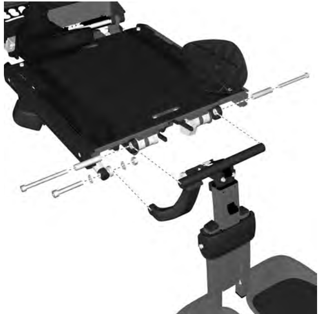
Figure 221. The legrest is held in place by two screws and spacers. The front bracket of the actuator is held in place by a screw and lock nut.
