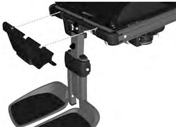
Figure 219. Remove the leg rest's top cover by carefully pulling it straight out.
