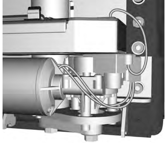
Figure 110. Disconnect the motor cable from the ICS-Master Module.
