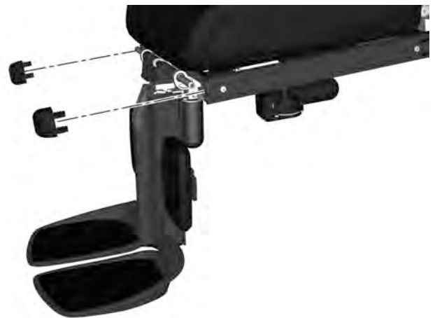
Figure 234. Remount the front ends of the UniTrack rails.
