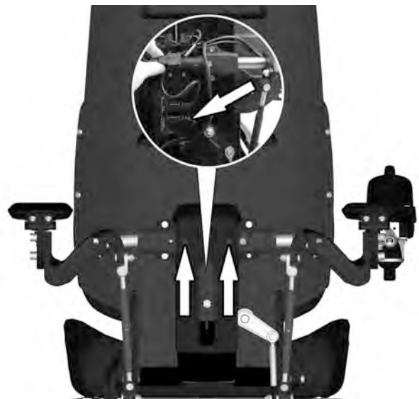
Figure 90. The contact block is located under the cover which is attached with two screws.
