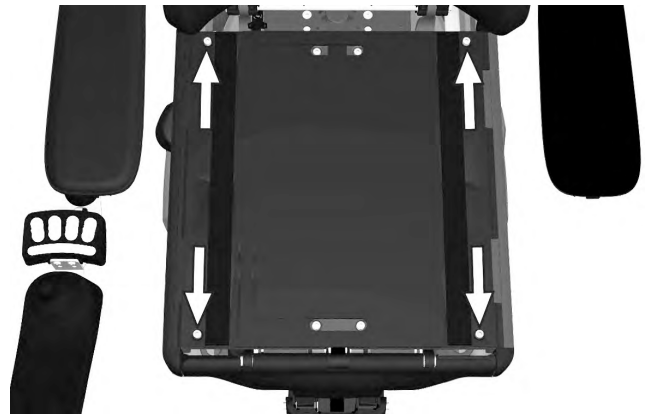
Figure 242. The seat plates are held in place by two screws at the back edge and two quick-mount clamps at the front.
