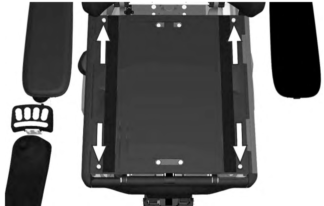
Figure 87. The seat plates are held in place by four screws.
