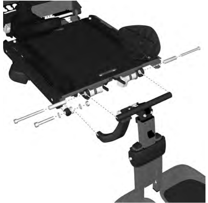
Figure 222. The legrest is held in place by two screws and spacers. The front bracket of the actuator is held in place by a screw and lock nut.
