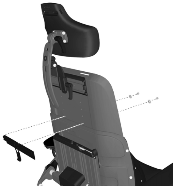
Figure 254. The locking mechanism is held in place by two screws.
