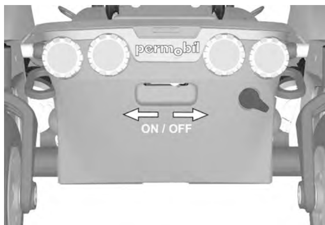
Figure 158. Circuit breaker/Battery isolator.
