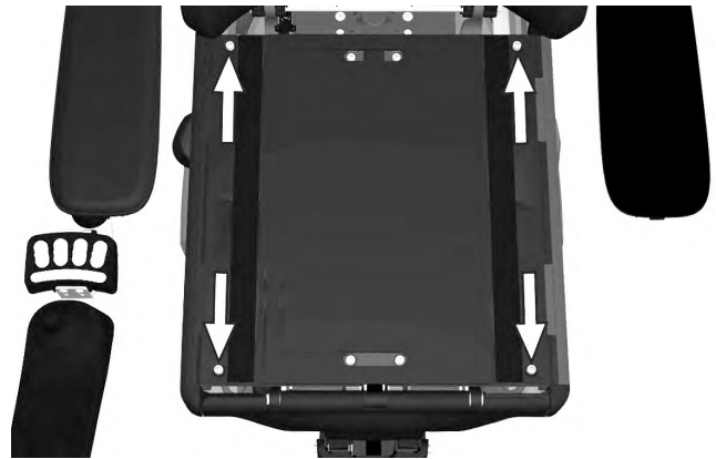
Figure 74. The seat plates are held in place by four screws.
