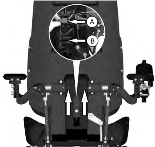
Figure 194. The plastic cover is fixed using two screws.
