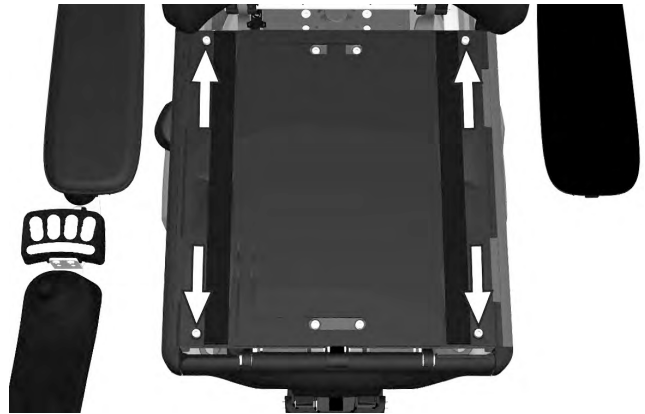
Figure 175. The seat plates are held in place by four screws.
