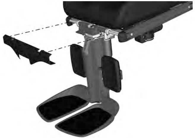
Figure 235. Mount the legrest's top cover by carefully pressing its bracket into place on the legrest's fixing screws/spacers.
