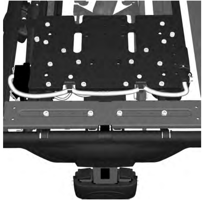
Figure 209. Backrest actuator cabling.
