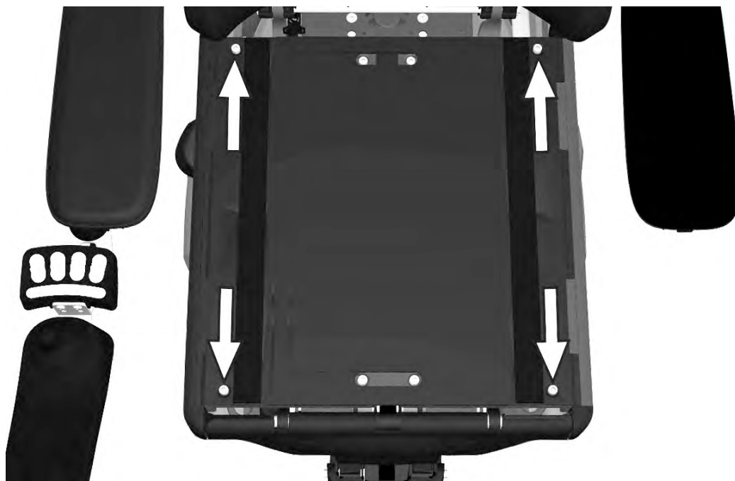
Figure 187. The seat plates are held in place by four screws.
