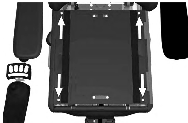
Figure 247. The seat plates are held in place by two screws at the back edge and two quick-mount clamps at the front.
