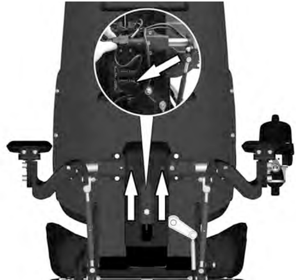
Figure 178. Disconnect the Rnet cable from the contact block at back of the back rest.
