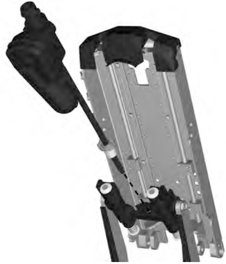
Figure 124. Remove the actuator from the sleigh by unscrewing its nut.
