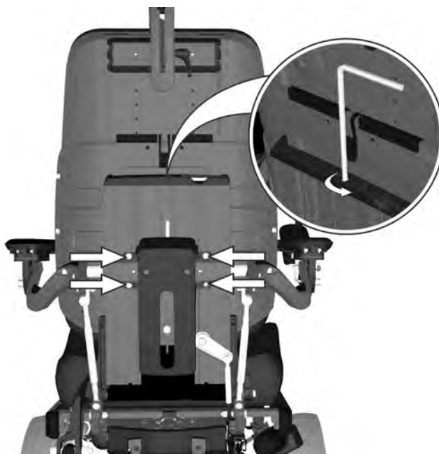
Figure 256. The armrest height is fixed using four screws. To perform this height adjustment, use the adjustment screw in the center of the backrest.
