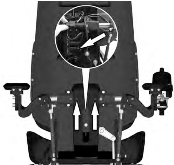
Figure 101. The contact block is located under the cover witch is attached with two screws.
