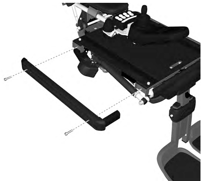
Figure 243. The UniTrack rails are fixed in place with two screws each.
