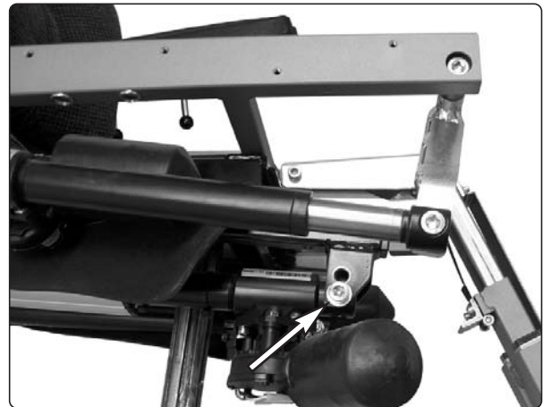
Fig. 33. Unfasten the front bracket on the seat tilt actuator.
