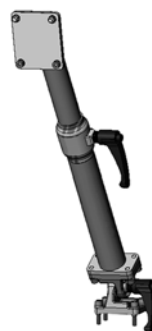
Figure 5. The upper locking lever holds the steering bar in place. The angle of the fixing tube is determined by the lower locking lever.
