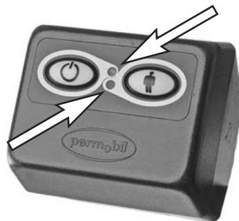
Figure 8. The two light diodes that indicate the Co-pilot's current status and also show errors.
