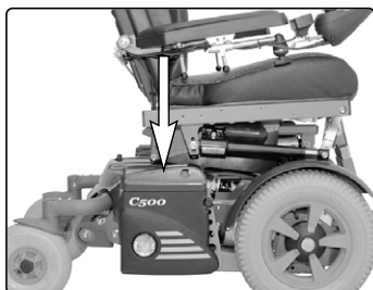
The Charging Fuse is located under the Main chassis cover
