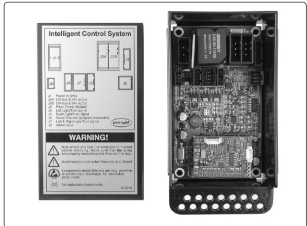
ICS master module with cover removed
