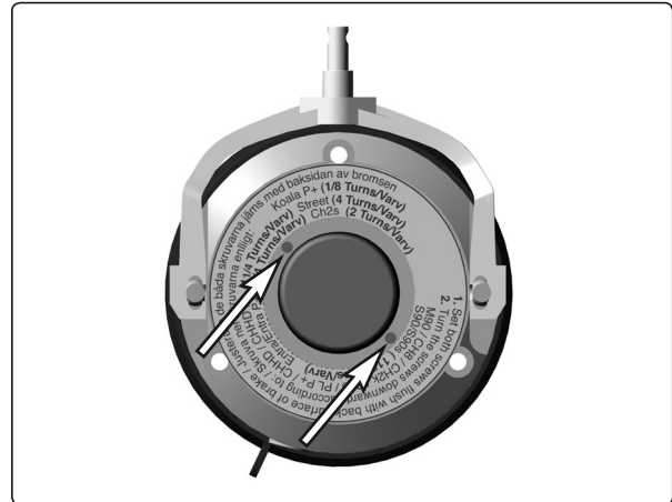
Wheel lock adjustment is made using the two adjusting screws.
