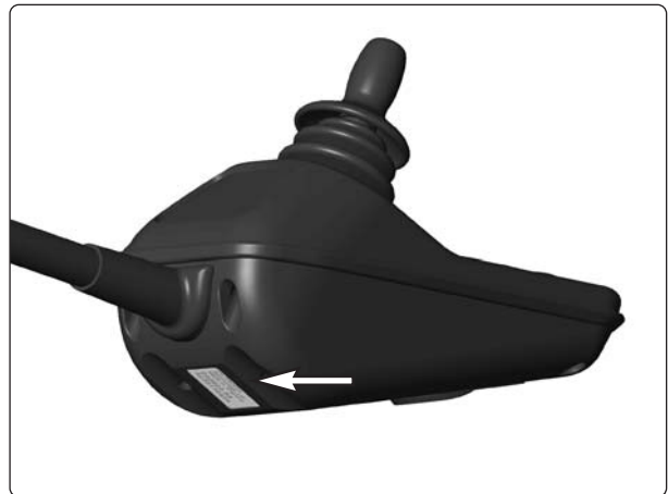
Control panel VSI identification number.
