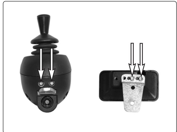
The Control panel and Seat control panel fixings.
