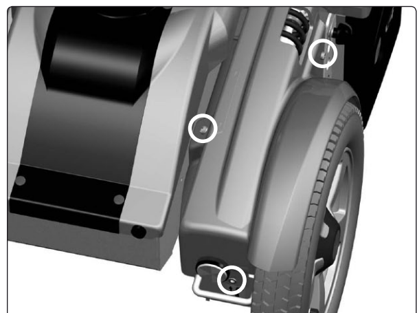
The front fender is mounted with three screws.
