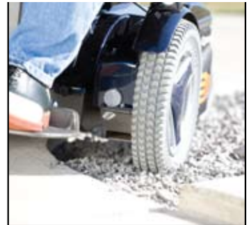
ESP (Enhanced Steering Performance) virtually eliminates the need for constant manual correction when driving on uneven ground, soft surfaces, angled and sloped areas or at high speeds.
