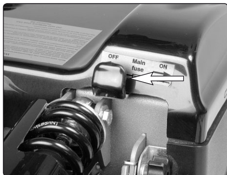
Main fuse in the OFF position.
