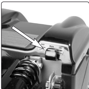
Lever for automatic main fuse
