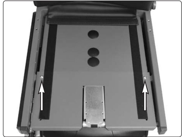
The seat plate for the Corpus seat is held in place with two screws.
