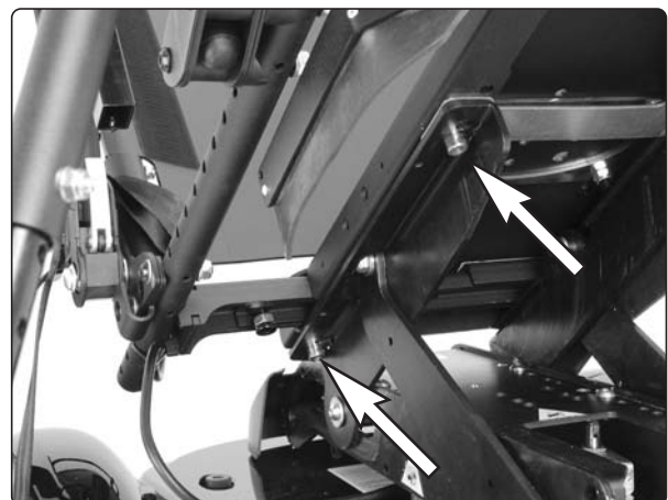
The seat is held in place with two screws on the left and right sides.
