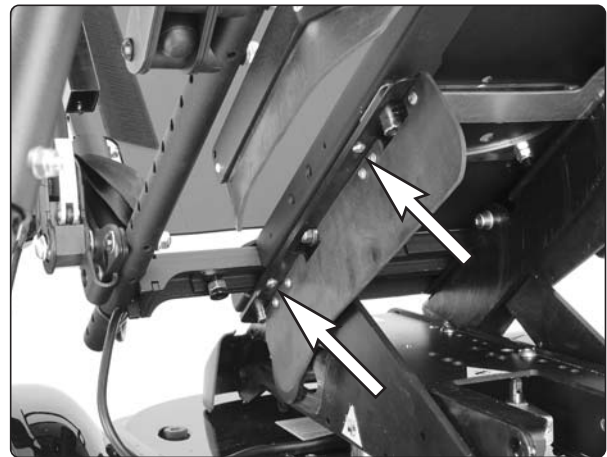
The crush protection devices on the left and right sides are held in place with two screws.
