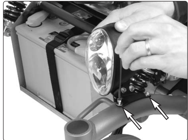
The front lights are fixed in place with two screws on each link arm.
