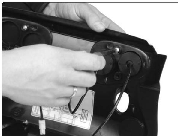
The rear lights are each held in place with two screws.
