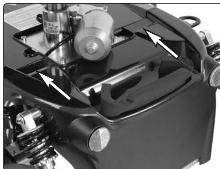
Position of the hook and loop fasteners.
