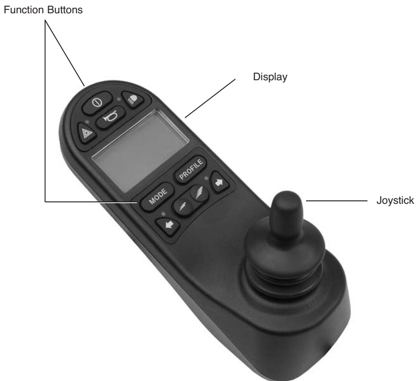
Control Panel Overview
