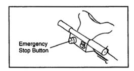
If it is necessary to use the Emergency Stop Button, ensure that Stair-Trac is examined by a qualified service person before it is used again.
