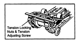
When decreasing tension, after turning the Adjusting Screw, press down on the tracks to remove any slack in them and to relocate the rear axle.
