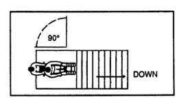
Note Page 14 Item 7 3. Keeping both hands on the hand grips, use your thumb to press the left side of the Operating Switch to move Stair-Trac forward. Release the Switch when the leading edge of the red "STOP" mark on the Drive Frame reaches the top of the stair nose.
