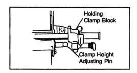
Close the Holding Clamps over the wheelchair handle, ensuring the Retaining Pin is on the outside of the Holding Clamp.
