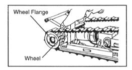
When re-installing the track, ensure the chalk mark you've made on the track lines up with the chalk mark on the wheel. Check track alignment as outlined at the beginning of this chapter.
