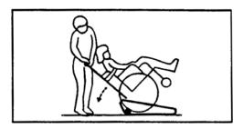
Pull the black Release Handle located just below the controls on the Support Handle. This lifts the Safety Bar. Then push the red Sliding Catch forward. Tip the Support Handle and wheelchair forward until the wheelchair touches the floor.
