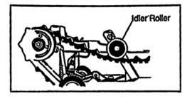
At a point halfway between the Idler Roller and the Drive Roller, press down firmly with your hand. At the closest point the track cogs should be 70mm  $\pm$  3mm (2 3/4 in  $\pm$  1/8 in) away from the part of the Drive Frame. You'll note that tracks will touch the motor housing, but is taken into consideration in the
