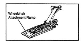
Attach the wheelchair as described under "Attaching Wheelchairs" on page 6, back the Stair-Trac away from the Ramp and proceed to the stairway. The Ramp can now be carried to the destination area.
