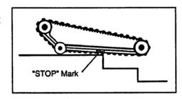
4. Keeping both hands on the Hand Grips, slowly tilt Stair-Trac forward until the tracks are resting on the stair noses, then press the left side of the Operating Switch to continue descending the stairs.
