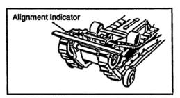
try re-positioning the track a few times to find a location that provides correct alignment.
