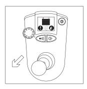
The wheelchair curves to the right driving backwards. (The curve's radius depends on the joystick's movement).
