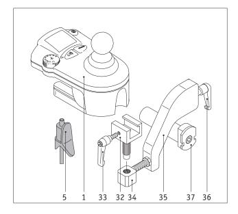
Dismantle the control unit in reverse order if it is to be used again directly by the wheelchair occupant. You can decide which of the individual components [32 - 36] should remain affixed to the wheelchair for use when the necessity arises.
