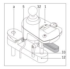
4.5.2 Mounting the control unit on the swivel arm
